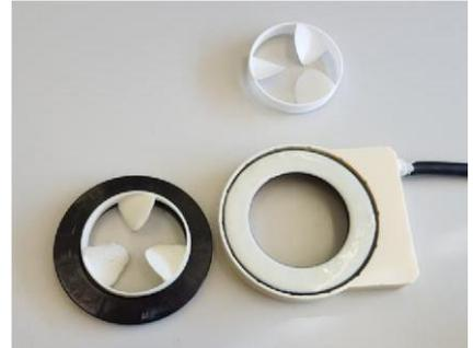
Place bottom ring on table, leave top ring in thruster. **Careful:** keep rings separate! Strong magnets!
