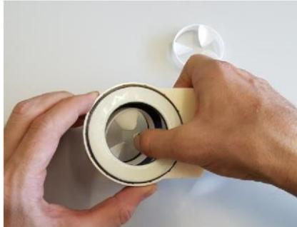
Lift thruster and gently push down against a propeller blade near the outer ring until bottom ring falls out.
