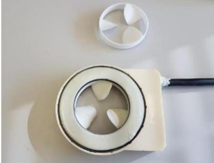
Place thruster on clean and non-magnetic surface, free of ferromagnetic objects or particles.
